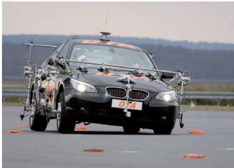
Picture 1: Vehicle manoeuvres: VDA obstacle avoidance test
