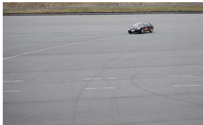
Picture 3: Steady-State Circular Test
